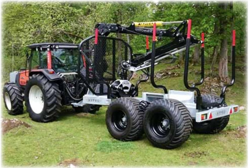
*A Cranab FC53DT with length of 8,5 meters is used as crane option.*
