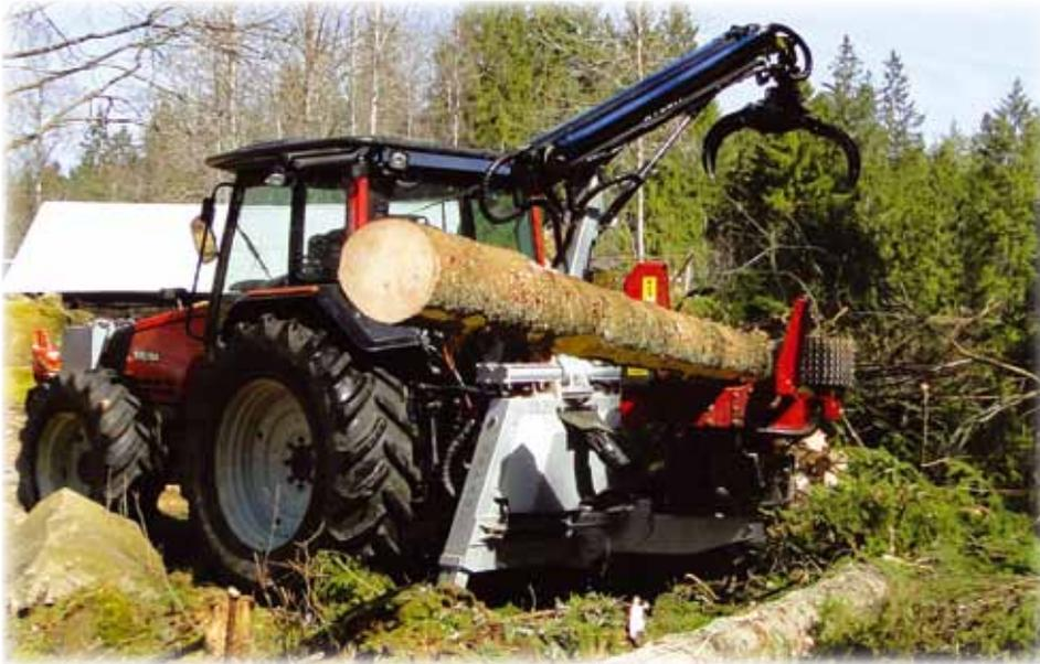
The HYPRO 755 is a generously equipped tractor-processor with a 7 metre crane. Processor and crane both have a working radius of 280 degrees, allowing felling on both sides.
