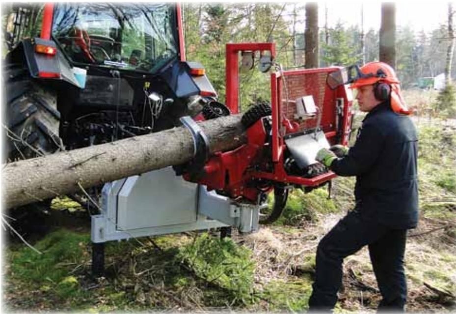
HYPRO 300 is a rational, quick, three point carried thinning processor which completes its tasks fast despite its small composition and light weight (700kg).
