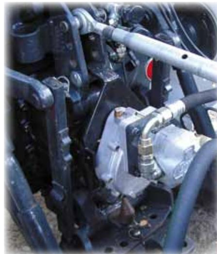
*The pump/gear unit is mounted directly on the power shaft of the tractor which gives lighter weight and a more compact montage.*
