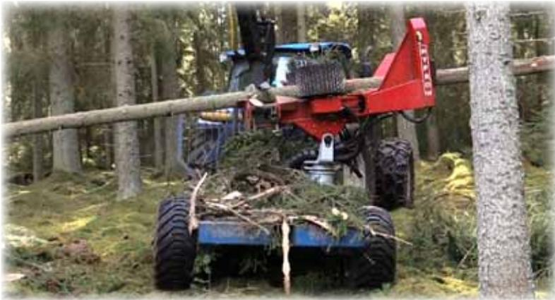
The **HYPRO 755 VB** is a trailer-mounted processor without crane, winch, pump or tank. It has been produced in order to combine a logging trailer with a crane and a processor, resulting in lower ground pressure and a lower purchase price.
