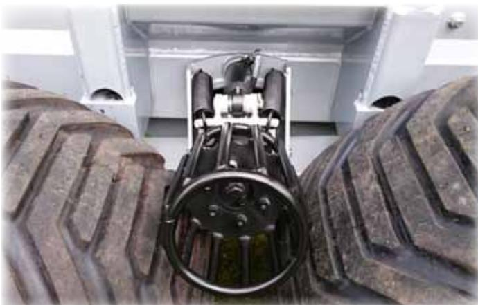
*On the HYPRO HV14 you have the option of choosing between robson drive or planetary gear. HYPRO 4WD robson drive provides high drive power and the drive unit is well protected*
