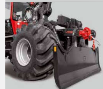
The 185 4-wheel Skidder have a hydraulically foldable clamping bench
